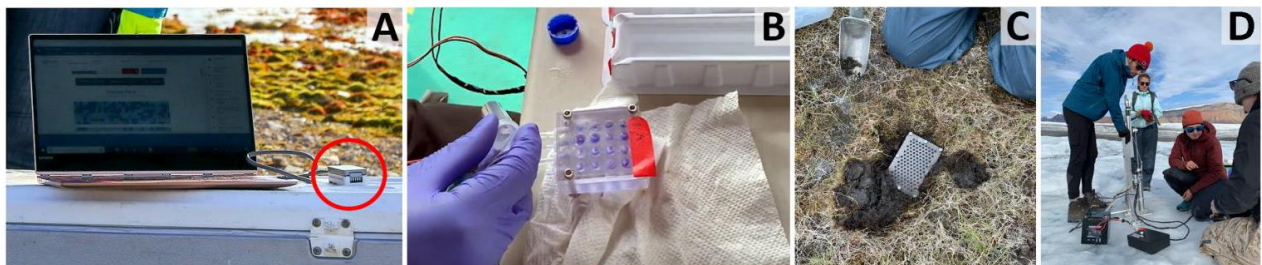
Figure 1: MICRO-life detection platform techniques employed in situ. A) Sequencing with MinION (red circle) at a High Arctic sampling site; B) \mu MAMA plate being used at McGill Arctic Research Station; C) Culturing with Cryo-iPlate in the High Arctic; D) Ice Drill on a sampling expedition.
