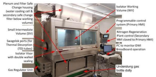
Fig. 1 Double Walled Isolator (DWI) Breadboard at the Space Research Centre, clean room University of Leicester.
